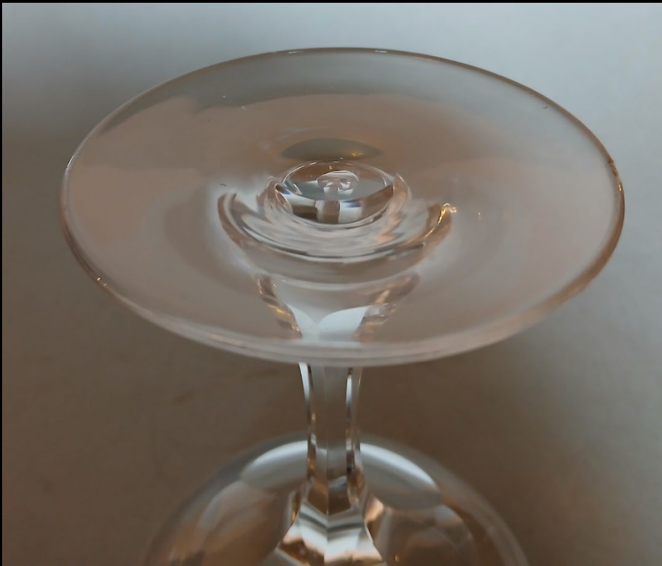
Left: Ground out pontil mark
