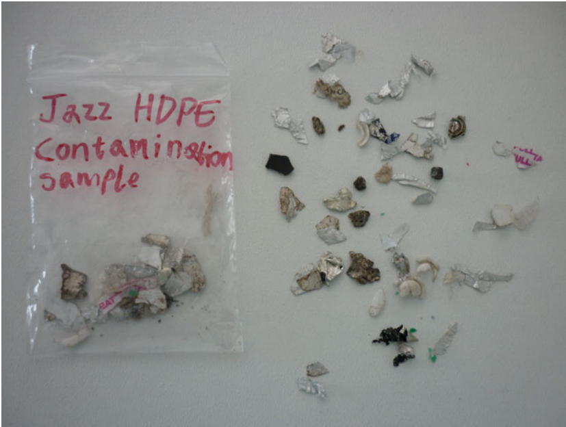
Contamination in HDPE granulate.
