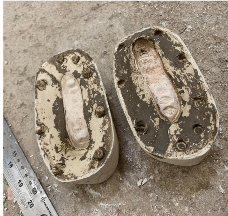
Trying some clay slip in the mold – this first pouring helps the mold to get the correct level of moisture for more successful casts afterwards.
