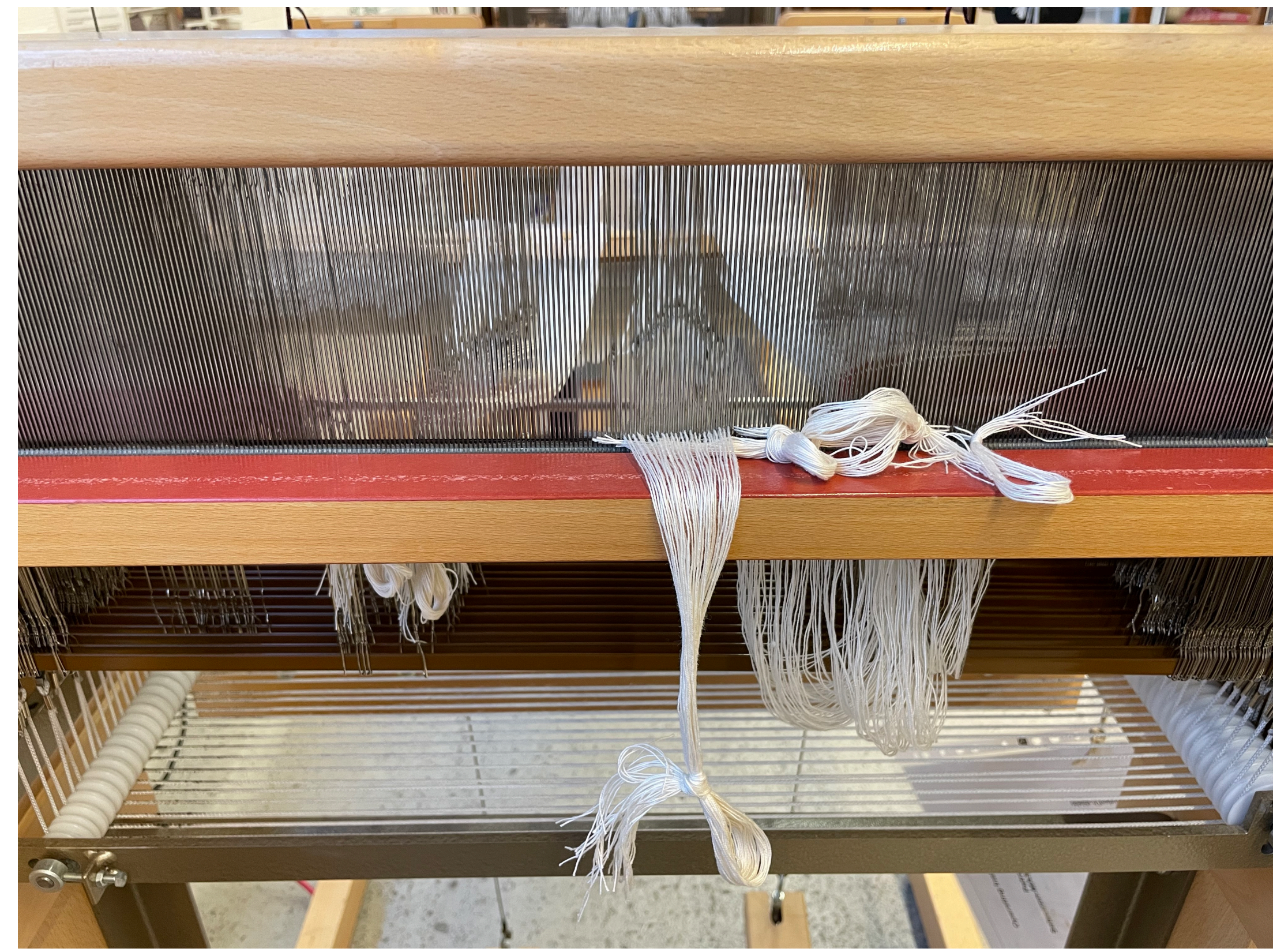
Reeding, Pulling 2 warp yarns through each dent in the reed as the pattern has 30 ends per inch and the reed has 15 dents in one inch.
