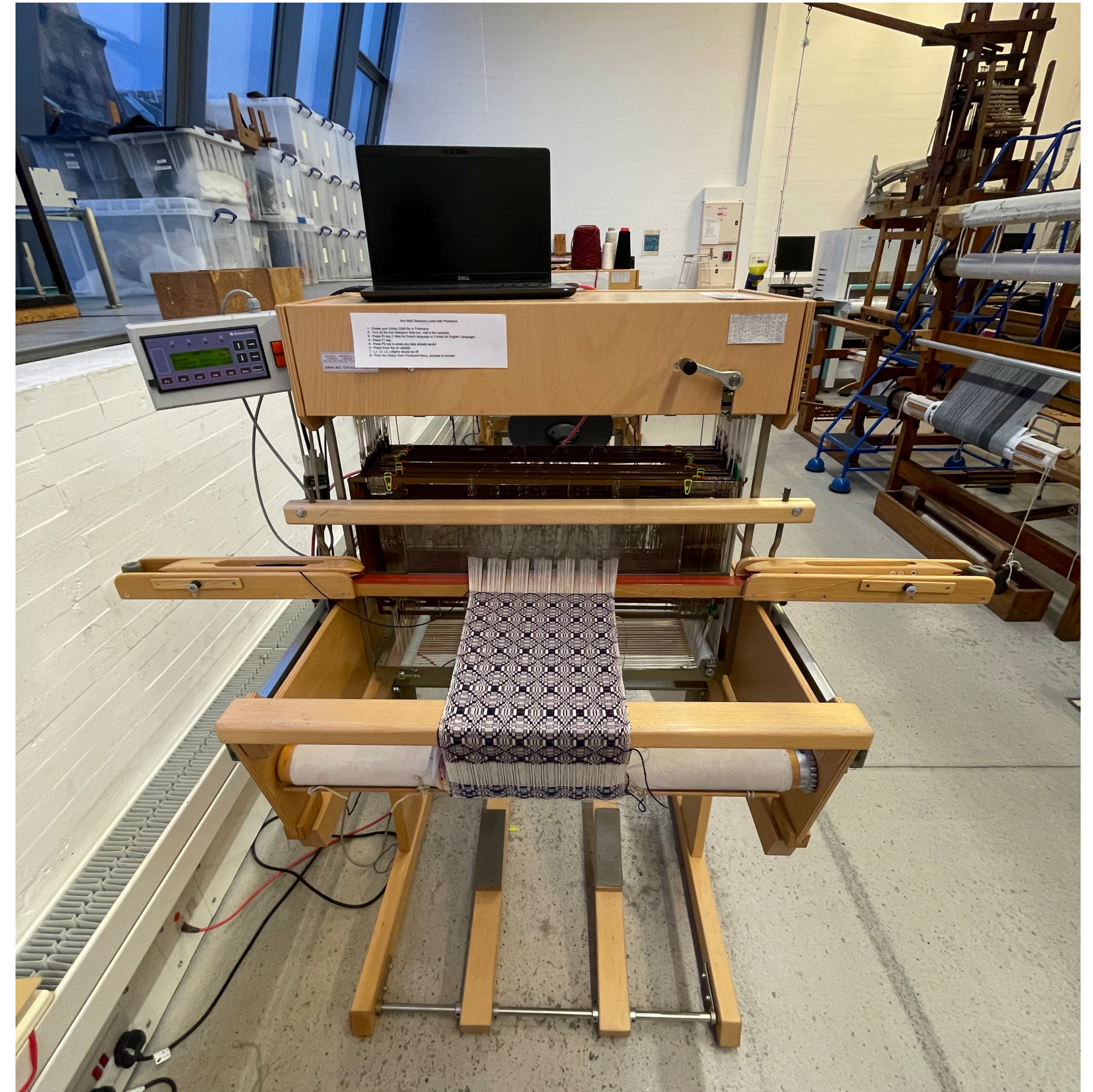
Figure 20: Weaving on the Swiss Arm Loom (Author's own, 2022)
