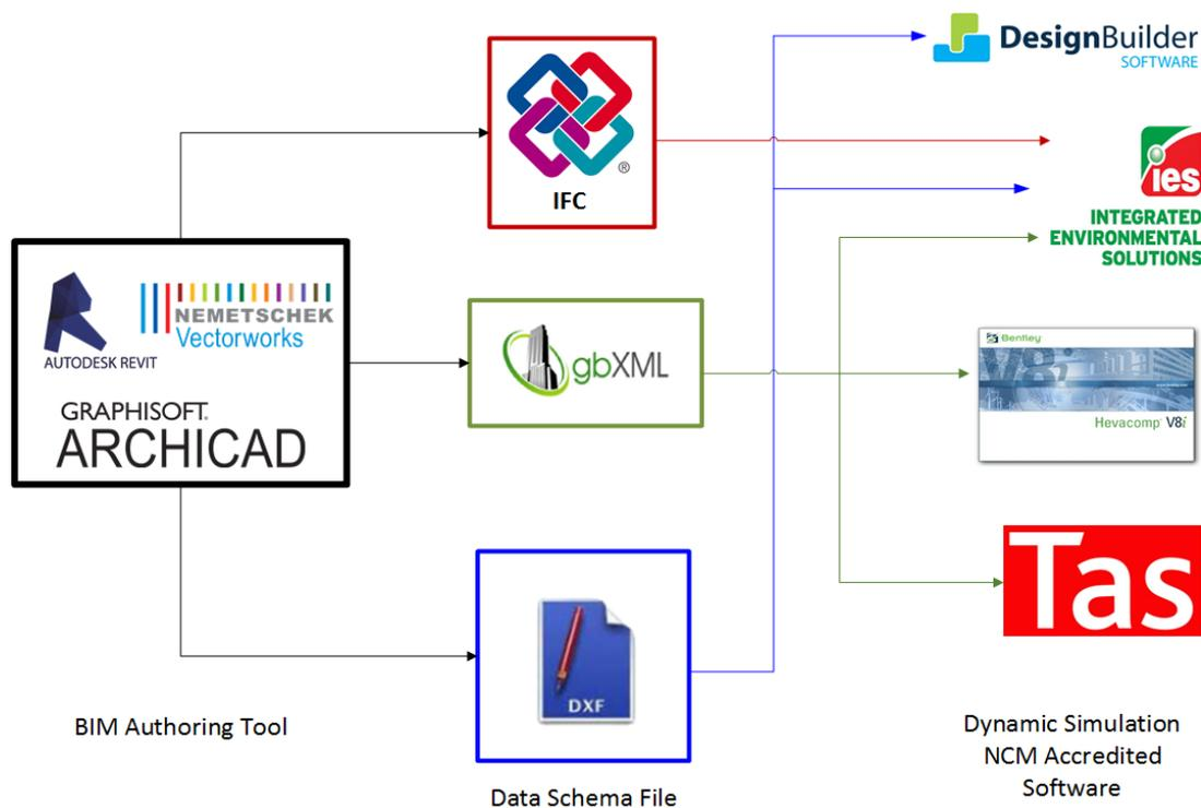
**Figure 5.4 Interoperability between BIM authoring tools and dynamic simulation tools (NCM Accredited)**
