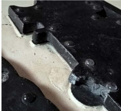
Figs 10 and 10a: Gowshall, 1933-46, the overlaid image suggests the company attempted to 'reflectorise' it almost as an after-thought, using miniature bullseye reflectors for the complex image.
