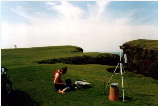
Measuring Rn fluxes, Calders Geo, Shetland
