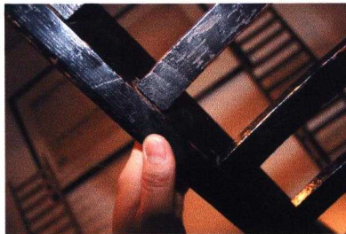
body of chair: ladderback ribs connections tongued and grove joints
