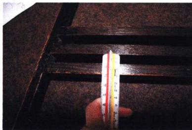
bracing support to the legs to stabilise the big chair.
