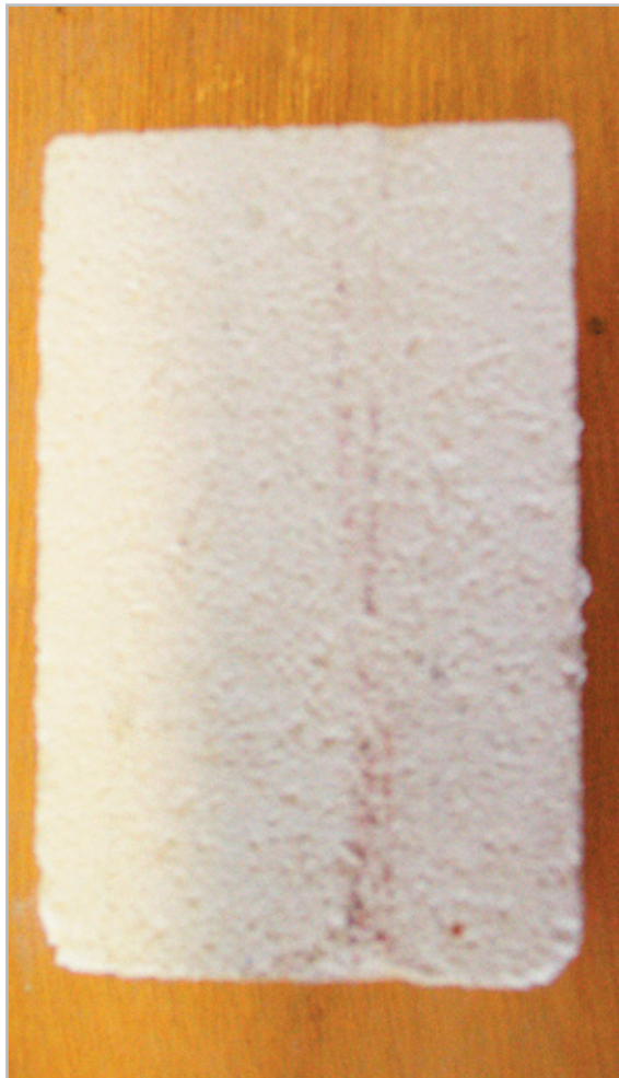
Fig.5.2h: Sample of ceramic materials, which sets at room temperature.
