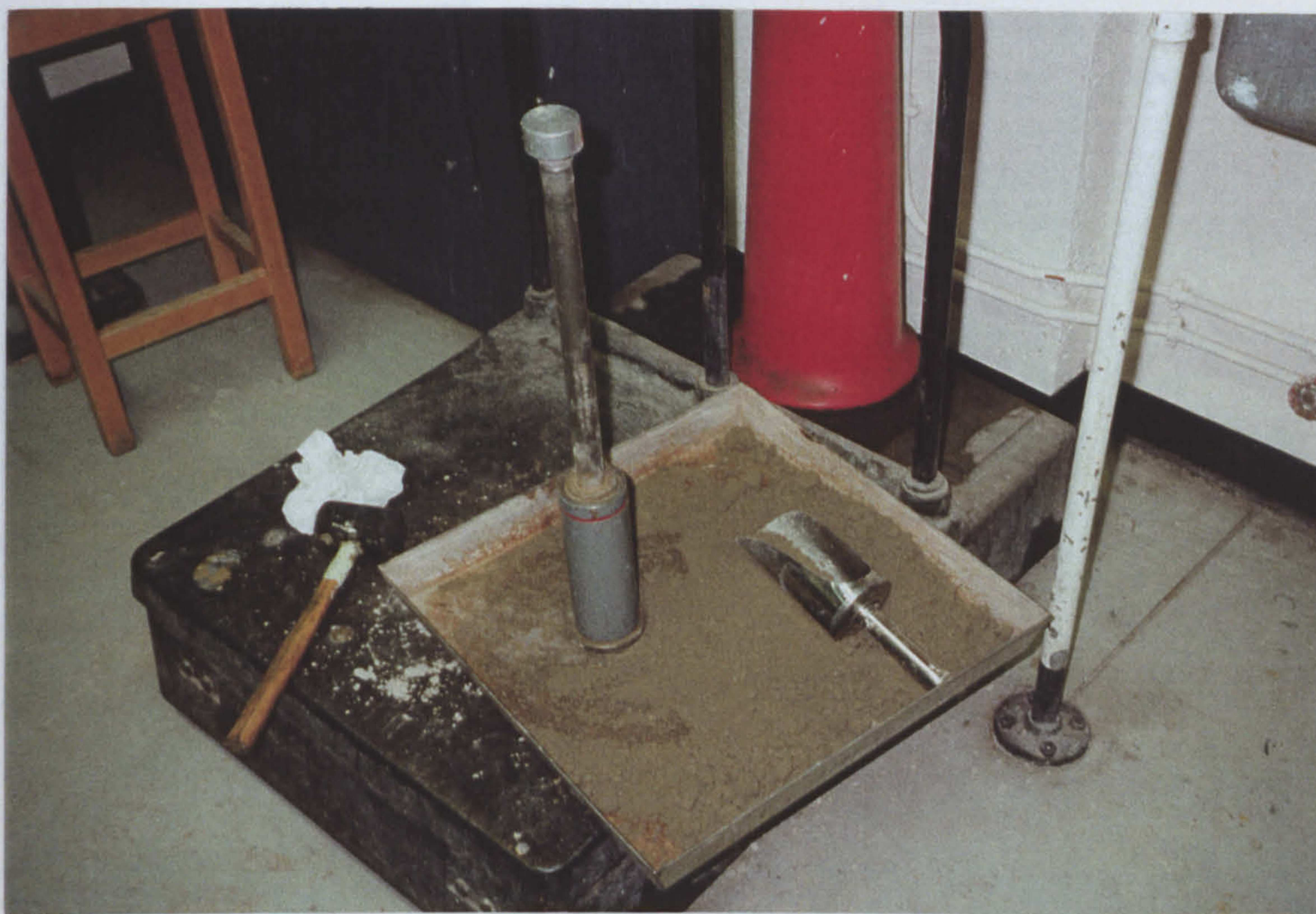
Mould used for producing the specimens (slightly compacted before applying actual compaction load)
