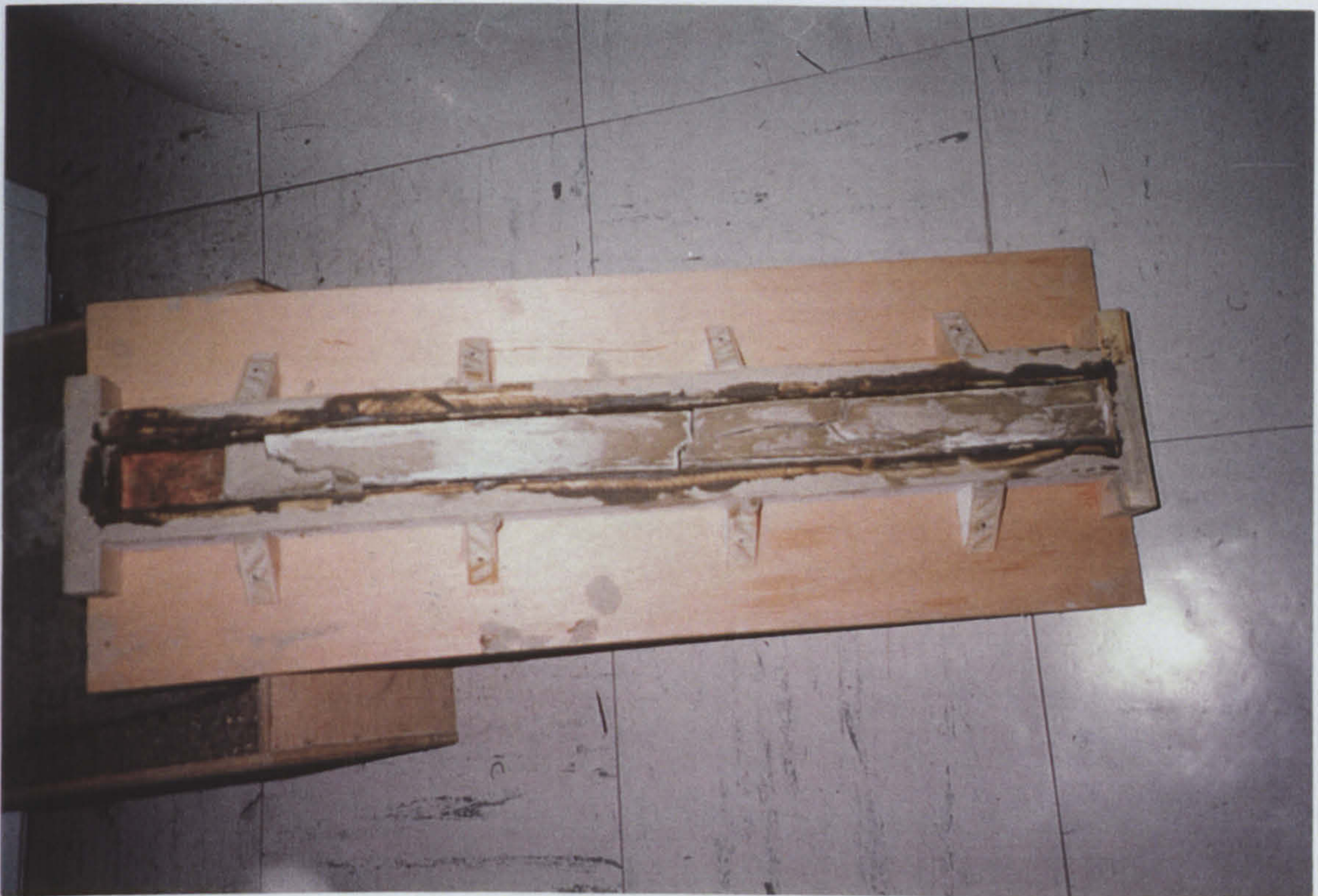
Wooden box used for linear shrinkage test (dry sample)
