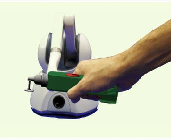
*'the stylus represents the polishing tool body with the polishing attachment sitting at a 90° angle from the end of the stylus'.*
