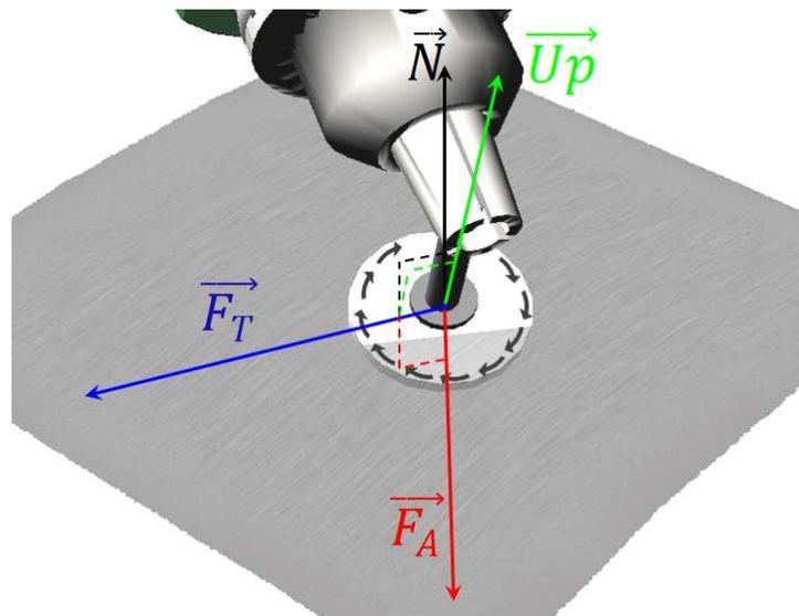
Figure 49. Modeling of the tangential force  $\vec{F}_T$  as a function of the estimated applied force  $\vec{F}_A$  and therefore of the normal vector  $\vec{N}$  at the contact point, and the vector  $\vec{U}_p$  on the  $y$  local axis of the haptic device.
