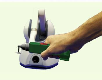
*'the stylus represents the polishing tool body with the polishing attachment sitting at a 90° angle from the end of the stylus.'*
