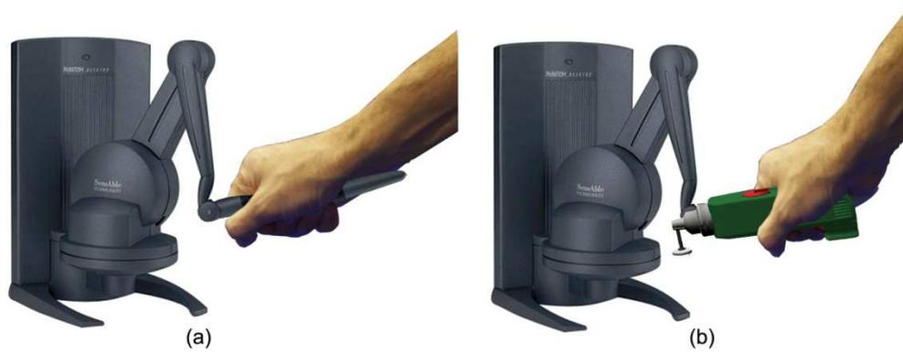
Figure 46. Handling of a Phantom Desktop as proposed in chapter 7, and mapping of the virtual precision rotary tool on the stylus of the haptic device (The body of the power tool in figure b. has been added with an image editing software).
