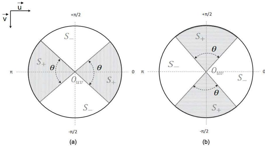
Figure 56. Circular sector areas  $S_+$  in which scratches are generated in the desired direction: (a) vertical and (b) horizontal. Sectors  $S_+$  are defined by a central angle  $\theta$  which has been heuristically set to  $80^\circ$  (Section 5.1.2.3).
