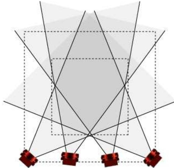
Figure 81. Volume capture composed by 4 cameras (<http://www.naturalpoint.com>).
