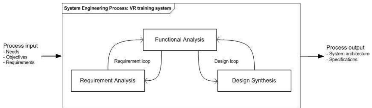
Figure 19. System engineering process which defined the methodology followed for the design of the VR training system (adapted from DAU Press, (2001)).
