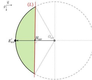
Figure 55. Case 3: representation of the circular segment area on the colour map. Percentages of task completion corresponding to pixels enclosed in that circular segment area are updated.
