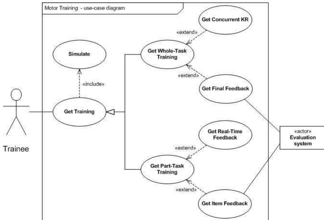
Figure 21. Use case diagram that describes the functionalities of the VR training system.
