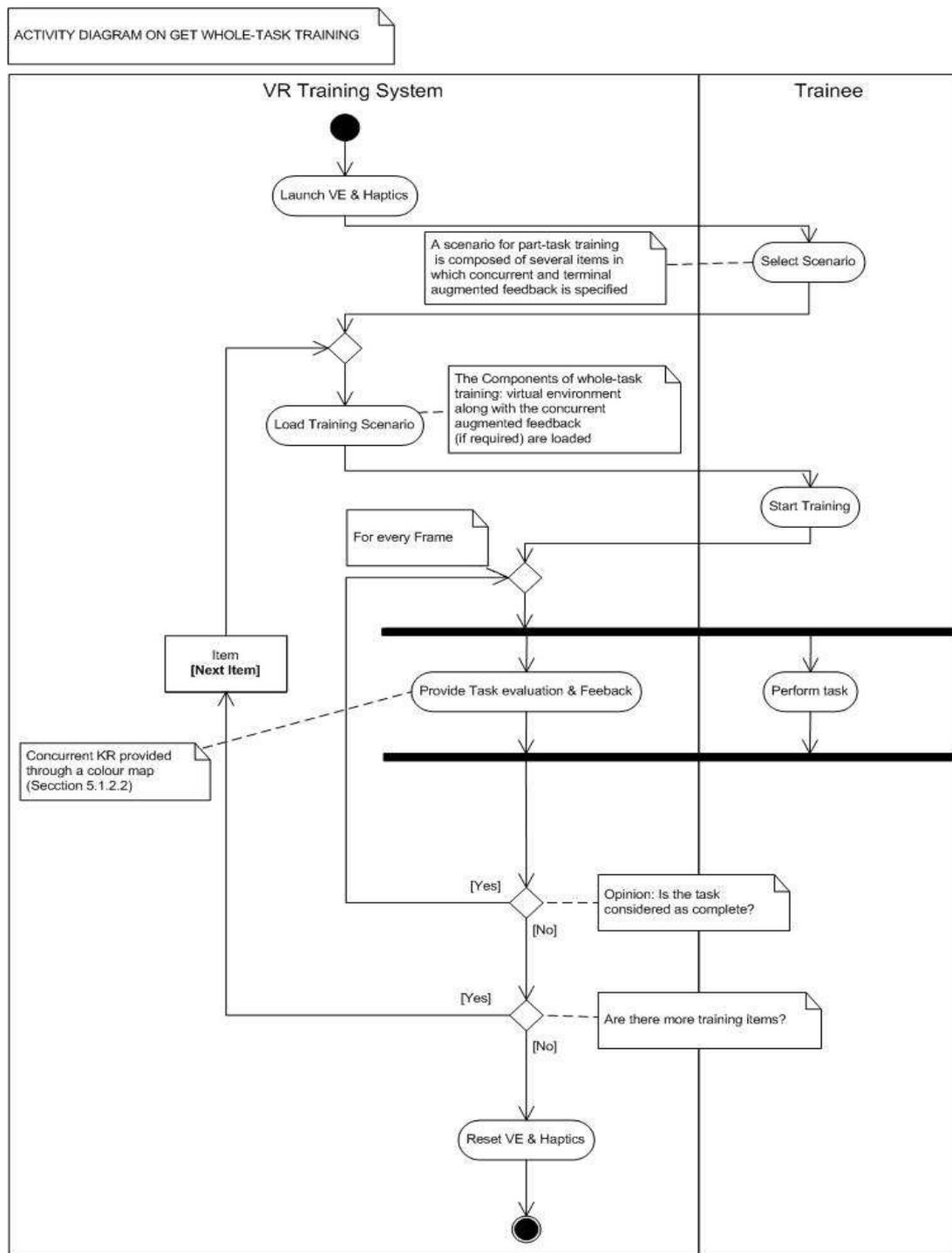
Figure 25. Activity diagram for the whole-task training method.
