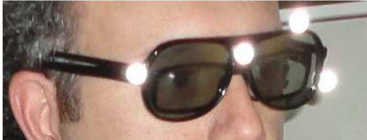
Figure 83. Passive stereoscopic glasses equipped with a set of infrared light reflective markers that form a unique rigid body for the tracking of the point of view.
