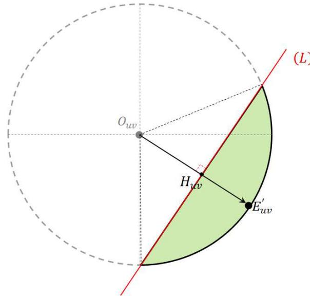
Figure 50. Representation of partial contact of the tool disc with the material surface on the colour map.
