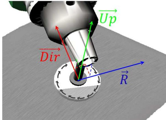
Figure 48. Local axes of the haptic device mapped on the virtual precision rotary tool.
