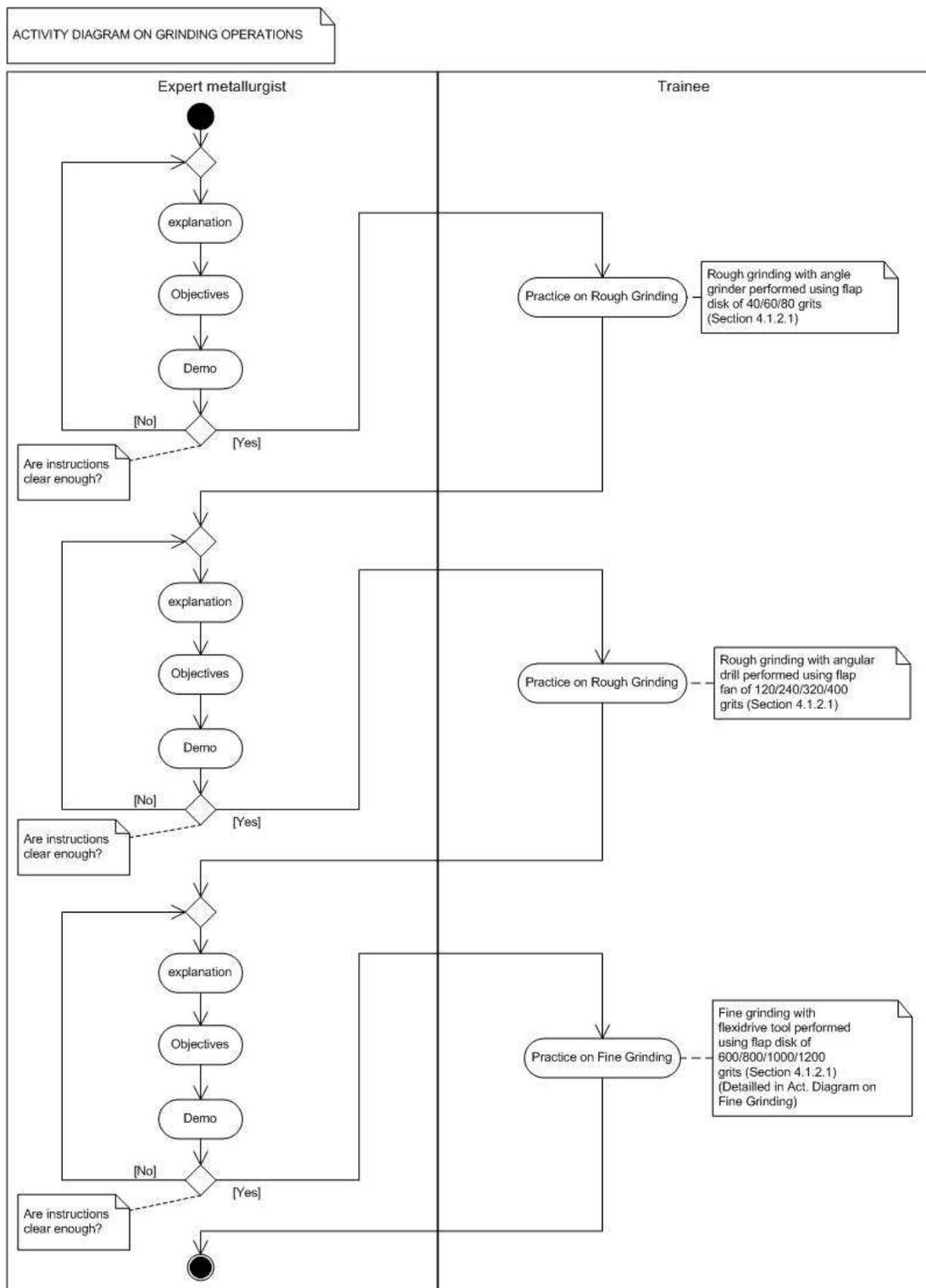
Figure 16. Activity diagram which depicts the workflow of activities between the expert metallurgist and the trainee during the training on grinding operations.
