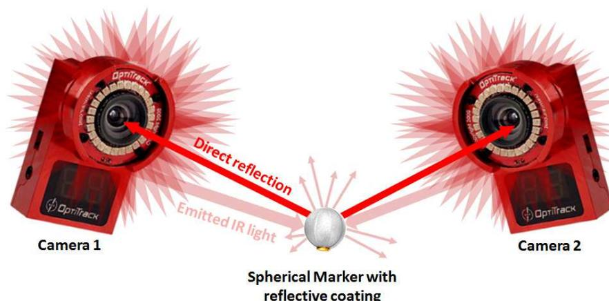
Figure 80. Example of tracking of a marker using two IR light emitted cameras
