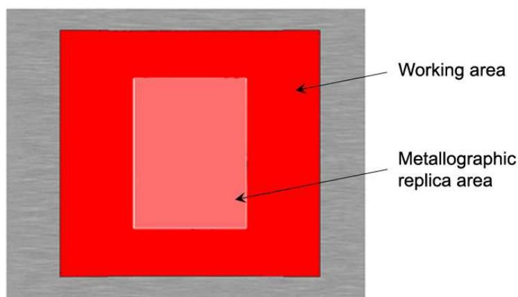
Figure 42. Colour map set on the material surface.
