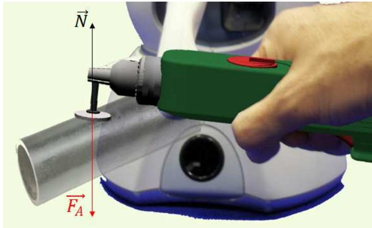
Figure 47. Representation of the estimated applied force  $\vec{F}_A$  on the material surface as a function of  $\vec{N}$ , the normal force at contact point.
