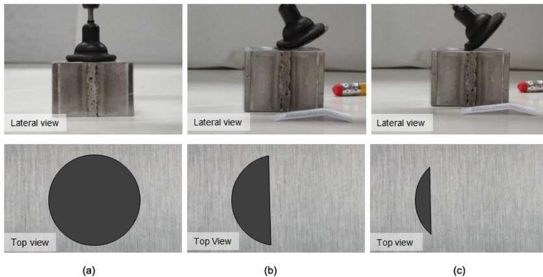
Figure 43. Tool disc when being pressed and inclined so it is (a) completely in contact with the material surface, and (b & c) partially in contact with the material surface.
