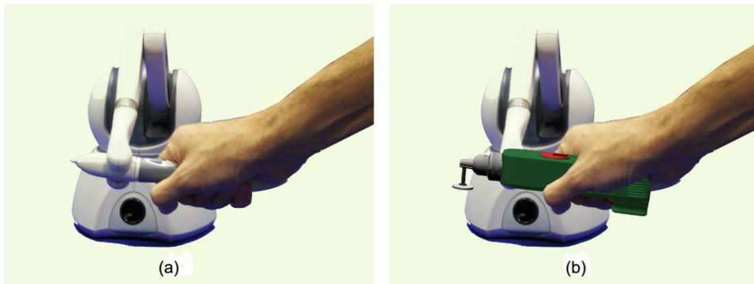
Figure 61. Handling of the haptic device and mapping of the virtual precision rotary tool on the device. The stylus represented the body of the virtual tool with the accessory attachment sitting at a 90° angle from the end of the stylus (This figure has been manipulated with an image editing software).
