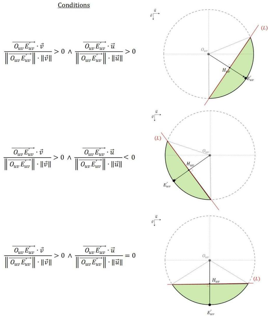
Figure 53. Case 1: representation of the circular segment area on the colour map. Percentages of task completion corresponding to pixels enclosed in that circular segment area are updated.
