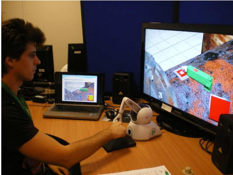
Figure 60. The haptic device was located in front of the monitor and instructions were displayed on a laptop placed on the left of the participant.
