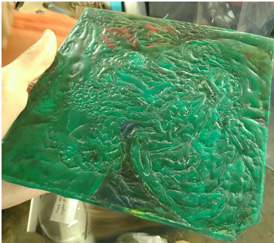
Figure 19: A beach-polymer tile with a flow-pattern surface created by melting it without pressing the top. Photograph. (Author's own, 2019)
