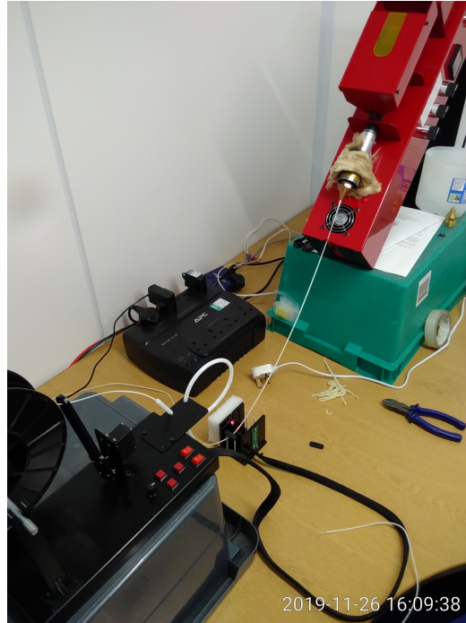
Figure 21: The Noztek Pro extruder in use with a filament winder produced by the same company, which repeatedly had blockages in winding. Photograph. (Author's own, 2019)
