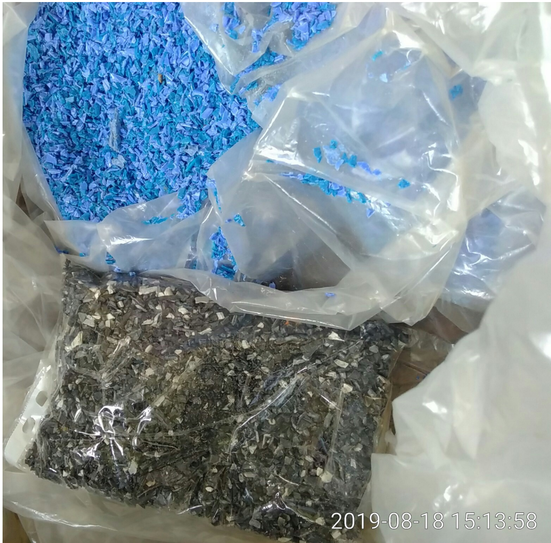
Figure 13: above: Plastic@Bay's beach-picked PP barrel granulate, below: post-WEEE ABS granulate from ROAR. Photograph. (Author's own, 2019)
