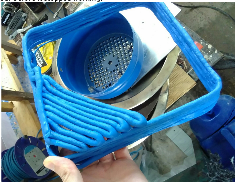
Figure 14: Aborted hand-guided tray extrusion. Photograph. (Author's own, 2019)
