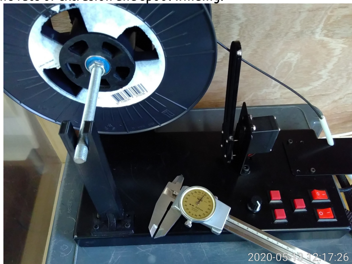
Figure 22: One example of the filament measured at 2.1mm. Photograph. (Author's own, 2020)
