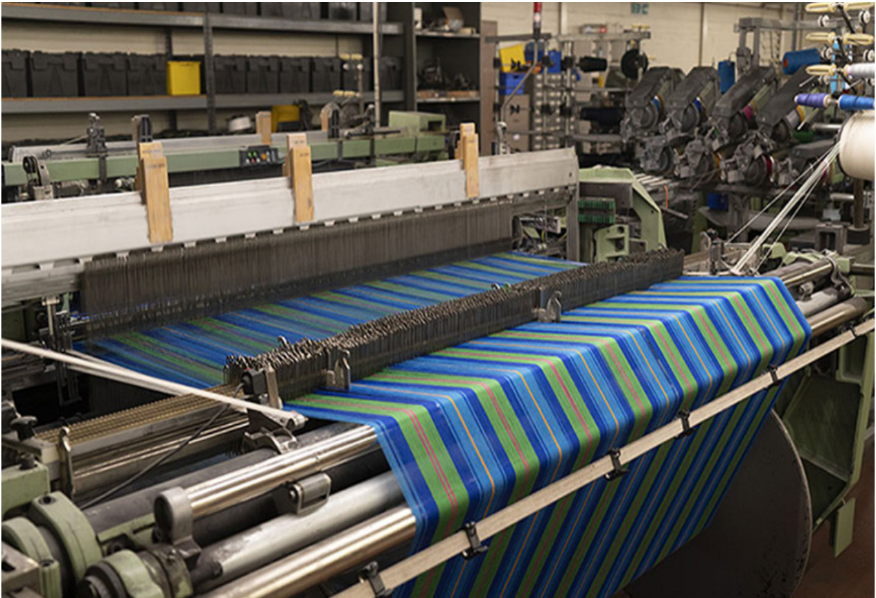
FIGURE 4: Rapier Loom. Locharron mill (2019).
