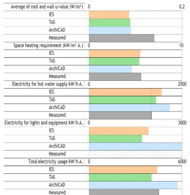
Figure 10: Comparison of predicted and measured energy use.
