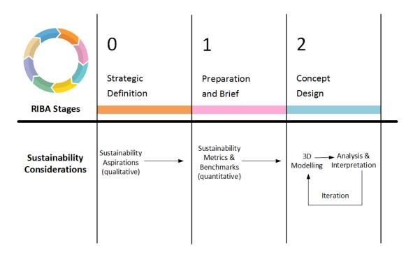
Figure 8.1 Sustainability definition aligned with the RIBA Plan of Work 2013
