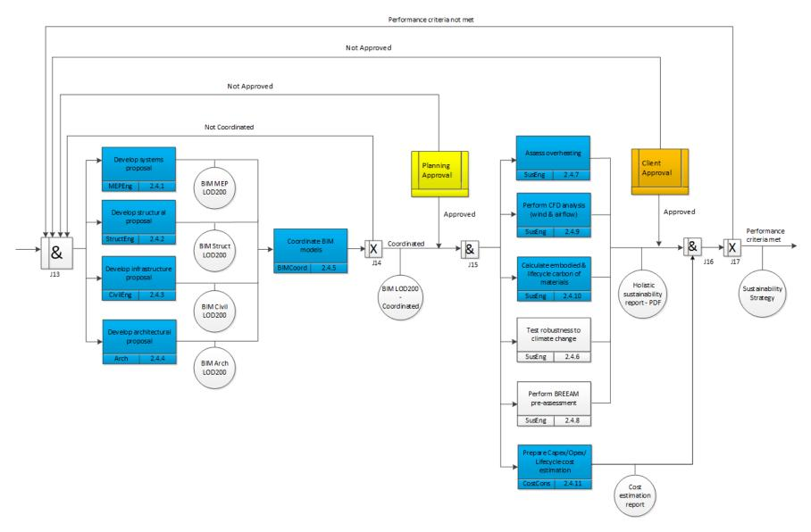
Figure 6.30 Amendments to UOB 2.4 "Develop holistic concept" decomposition based on unstructured descriptions [White UOBs]
