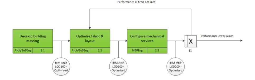
Figure 6.8 High-level decomposition IDEF3 diagram of Stage 2 "Develop Concept design" [Green UOBs]
