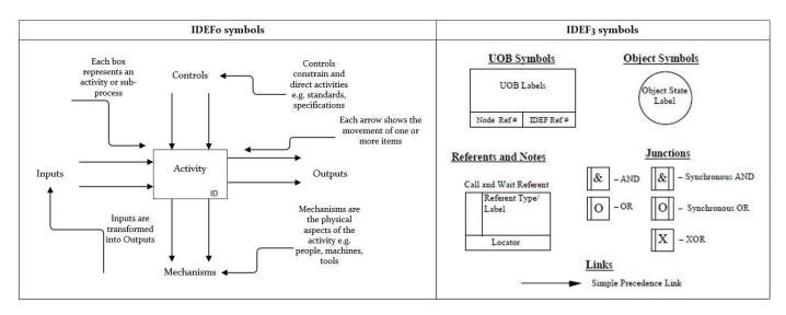
Figure 1 Symbols used for process description schematics
