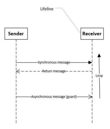
Figure 4.7 UML Sequence Diagram notation (adapted from OMG, 2011)
