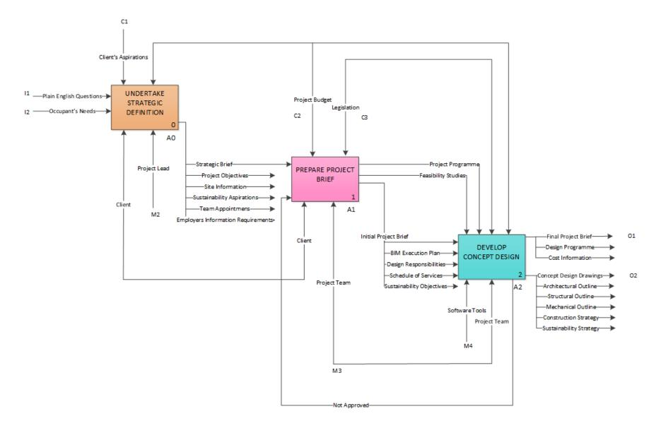
Figure 6.1 High-level IDEF0 decomposition diagram
