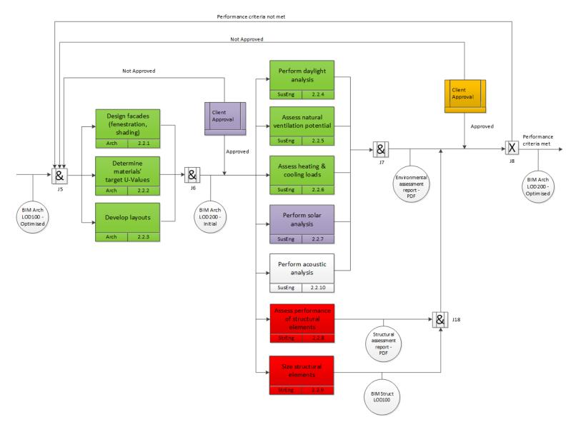
Figure 6.20 UOB 2.2 "Optimise fabric and layout" decomposition amended according to Narrative 10 [Red UOBs]
