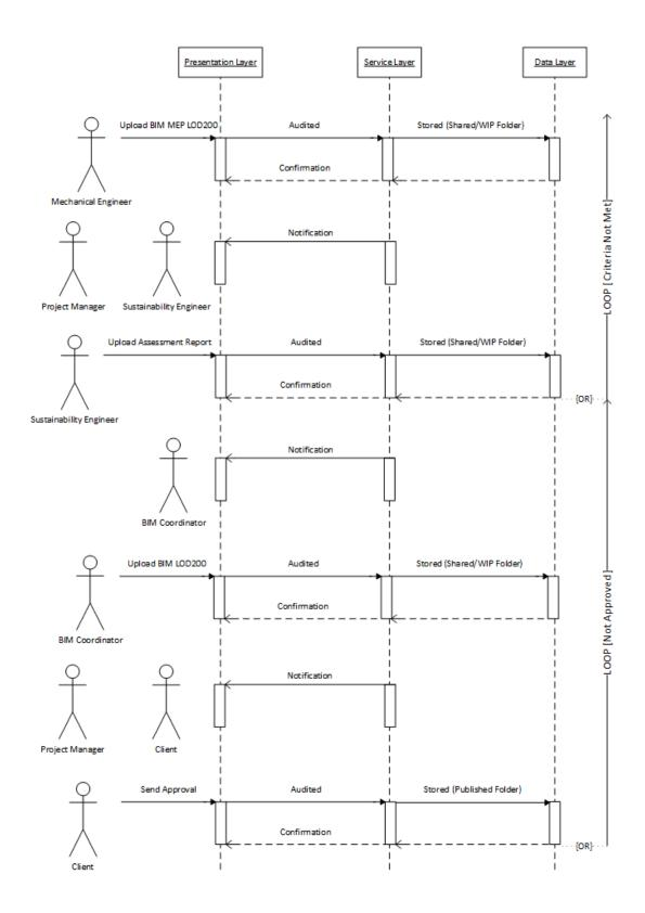
Figure 6.43 Use Case Scenario 4 – Mechanical Services [UOB 2.3] (Phase 1)
