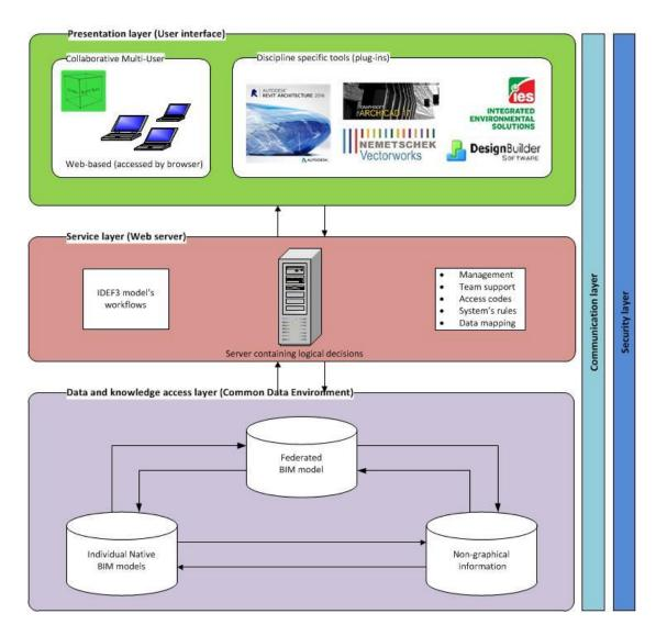
Figure 6.35 Green BIM Box – three-layered system architecture
