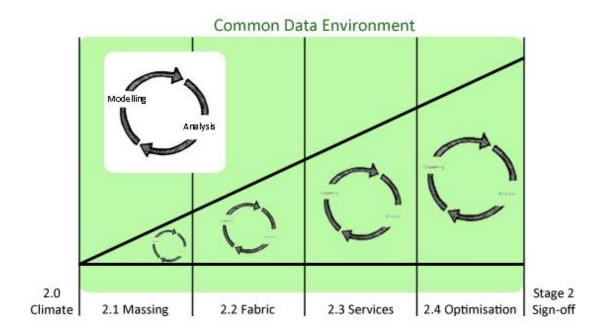
Figure 8.2 Soft-gates and assessment loops for SBD during Concept Design (RIBA stage 2) development
