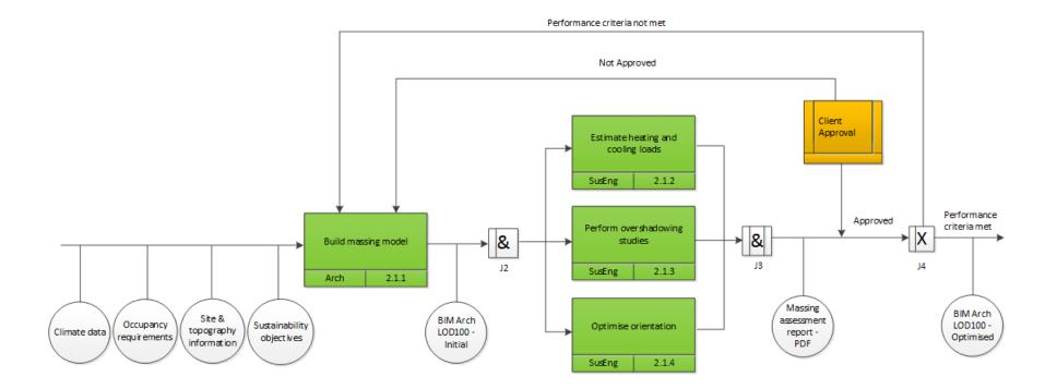
Figure 6.17 UOB 2.1 "Develop building massing" decomposition amended according to Narrative 7 [Orange UOBs]
