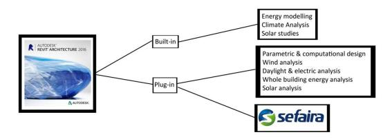
Figure 5.3 Revit 2016 rapid performance analysis capabilities
