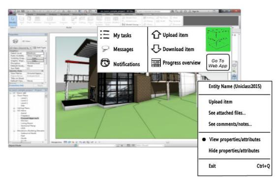
Figure 18 Plug-in presentation layer of the mock-up application (Revit)
