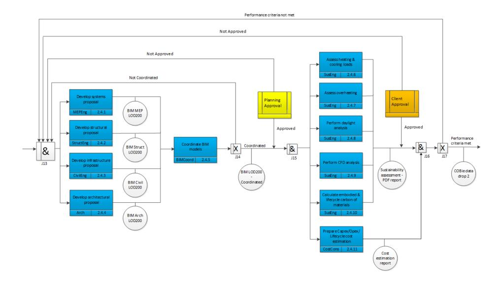
Figure 6.21 UOB 2.4 "Develop holistic concept" decomposition amended according to Narrative 10 [COBie data drop]
