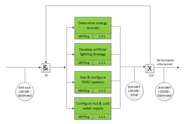
Figure 6.11 Decomposition of UOB 2.3 "Configure mechanical services" [Green UOBs]
