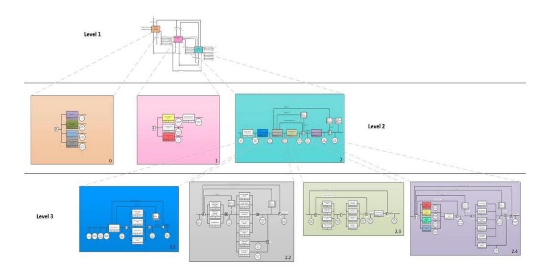
Figure 2 IDEF process model master-map showing hierarchical relationships between processes and their sub-processes (see Table 1 for detailed decompositions)
