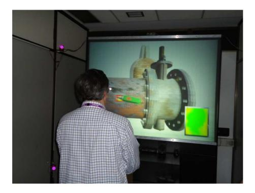
Figure 72. A trainee performs a whole-task training session, using the colour map on the metallographic replica area along with the magnification represented in the lateral window.
