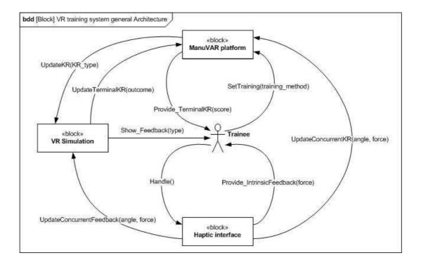
Figure 20. Block diagram of the general architecture of the VR training system which enable part-task and whole-task training and can provide concurrent and terminal augmented feedback; and a representation of the interaction between all the actors involved in the proposed VR training.
