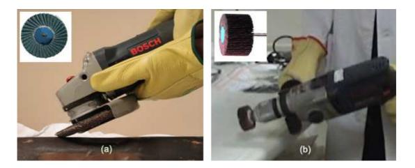
Figure 10. (a) Angle grinder equipped with abrasive flap disc of rough grits and (b) angle drill mounted with abrasive flap fan to perform rough grinding operations.
