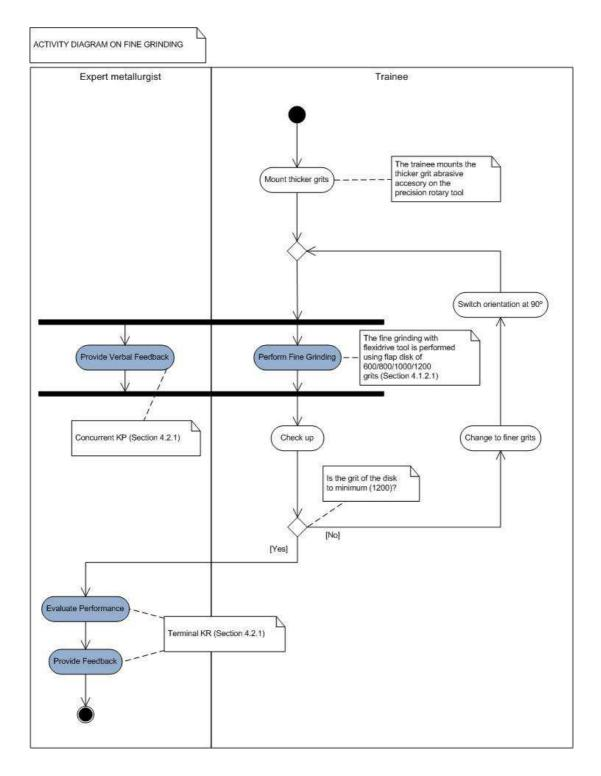
Figure 17. Workflow of activities conducted during conventional training on fine grinding operations. Highlighted activities related to task performance and information feedback are supplemented by the VR training system (Section 4.3).
