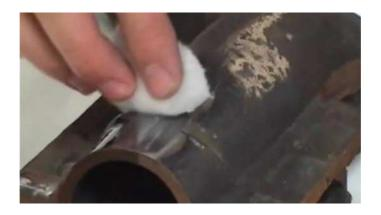
Figure 13. The etching process
