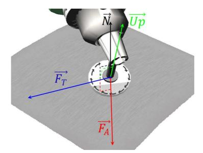
Figure 49. Modeling of the tangential force  $\overrightarrow{F_T}$  as a function of the estimated applied force  $\overrightarrow{F_A}$  and therefore of the normal vector  $\overrightarrow{N}$  at the contact point, and the vector  $\overrightarrow{Up}$  on the y local axis of the haptic device.
