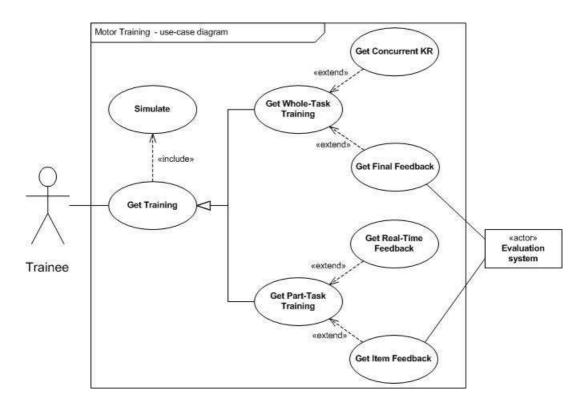
Figure 21. Use case diagram that describes the functionalities of the VR training system.
