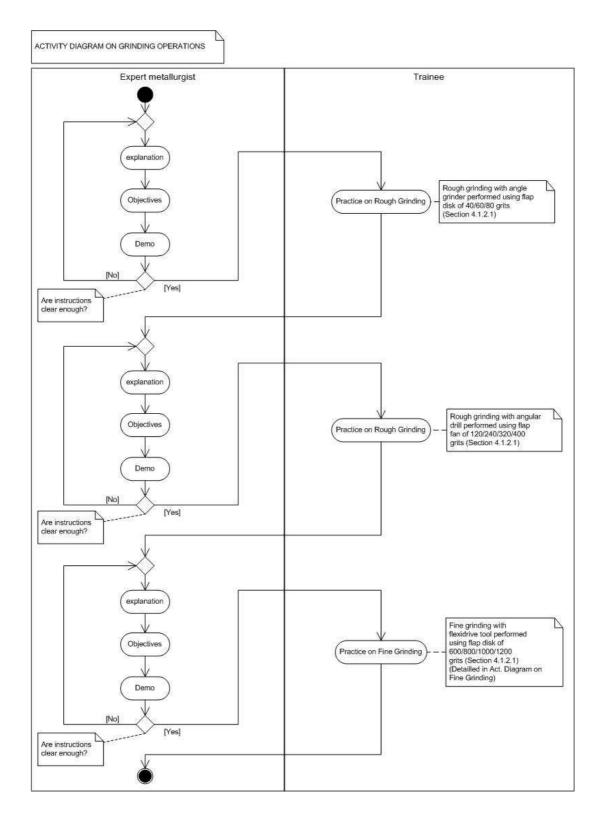
Figure 16. Activity diagram which depicts the workflow of activities between the expert metallurgist and the trainee during the training on grinding operations.
