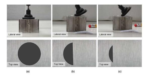
Figure 43. Tool disc when being pressed and inclined so it is (a) completely in contact with the material surface, and (b & c) partially in contact with the material surface.
