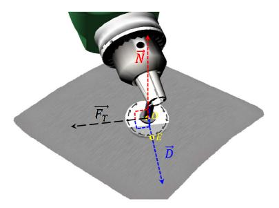
Figure 51. Determination of the point E on the tool disc.
