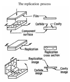
Figure 14. Schema of the replication process which records the topography of a material surface as a negative relief on a replica (Gandy & Findlan, 1996).
