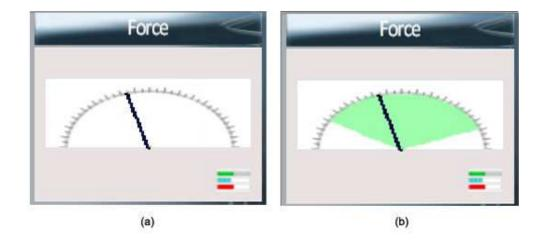
Figure 34. Dial indicator for force skill with (a) no reference of correctness to indicate targeted force and with (b) a green area to show the range for force skill.
