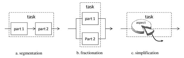
Figure 4. Three techniques for part-task training (segmentation and fractionation techniques appeared as proposed by Roessingh et al. (2002))
