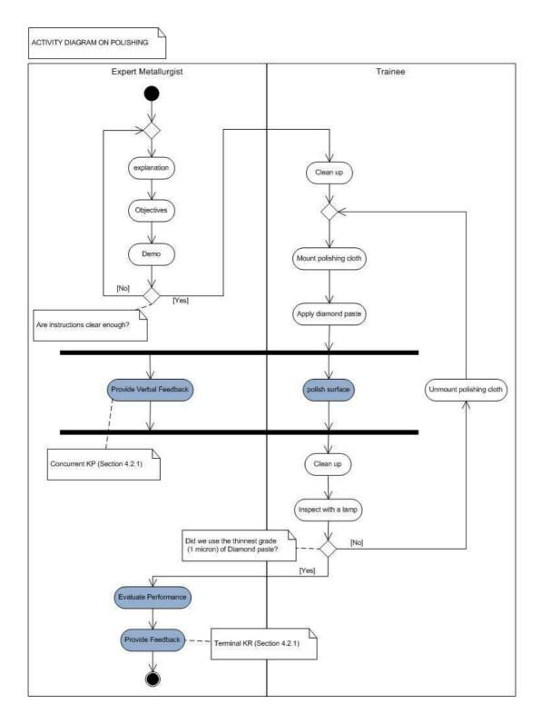
Figure 18. Workflow of activities conducted during conventional training on polishing operations. Highlighted activities related to task performance and information feedback are supplemented by the VR training system (Section 4.3).
