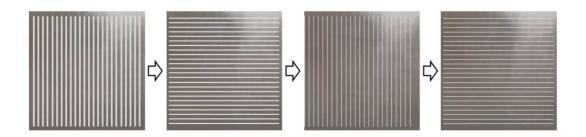
Figure 9. Sequence of grinding operations alternating the grinder orientation by 90° in order to remove scratches previously generated, with thinner scratches of perpendicular direction.
