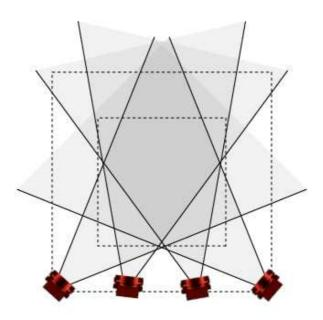
Figure 81. Volume capture composed by 4 cameras (http://www.naturalpoint.com).
