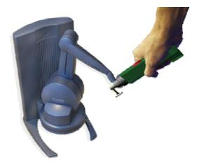
Figure 68. Mapping of the virtual precision rotary tool on the Phantom Desktop stylus (This figure has been manipulated with an image editing software).
