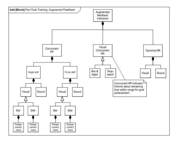
Figure 30. Configuration of augmented feedback indicators in part-task training<sup>4</sup>.
