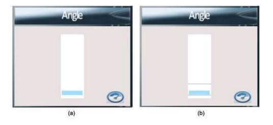
Figure 31. Bar indicator for angle skill with (a) no reference of correctness to indicate targeted angle and with (b) two grey lines to mark the boundaries of the range for angle skill.
