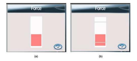
Figure 33. Bar indicator for force skill with (a) no reference of correctness to indicate targeted force and with (b) two grey lines to mark the boundaries of the range for force skill.
