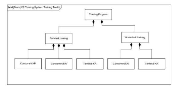
Figure 27. The VR training system enables carrying out the VR training suggested through a training program built with the training toolkit. Training programs encompass part-task and/or whole-task training throughout which augmented feedback can be provided.
