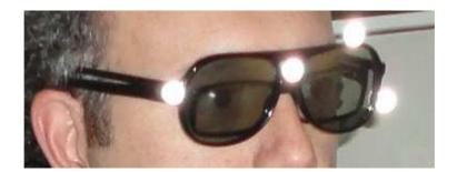
Figure 83. Passive stereoscopic glasses equipped with a set of infrared light reflective markers that form a unique rigid body for the tracking of the point of view.
