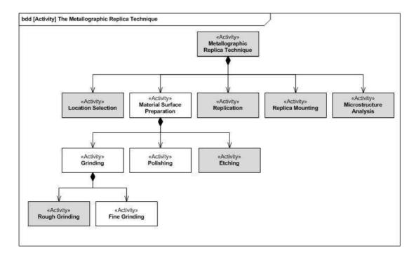
Figure 7. Stages of the metallographic replica technique with emphasis on fine grinding and polishing operations commonly carried out for material surface preparation (diagram resulting from discussions with two expert metallurgist from Tecnatom S.A.).
