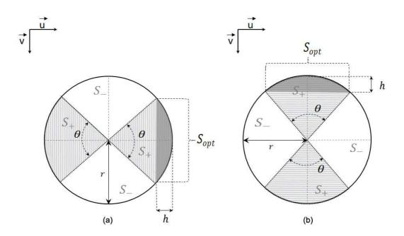
Figure 59. Definition of the optimum contact area so that all scratches are generated with the desired direction: (a) vertical and (b) horizontal with regards to the orientation of the metallographic replica area.
