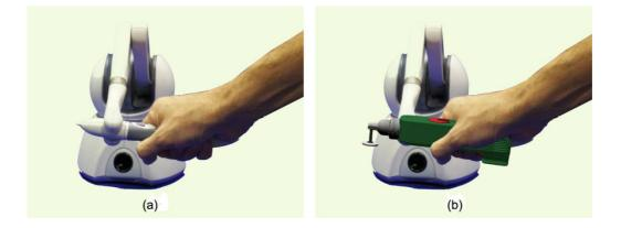
Figure 45. Handling of a Phantom Omni as proposed in chapter 6, and mapping of the virtual precision rotary tool on the stylus of the haptic device (The body of the power tool in figure b. has been added with an image editing software).
