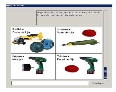
Figure 86.The GUI for the procedural training in the ManuVAR platform (the trainee is required to click on the picture which shows the tool and the abrasive accessory required to remove the oxide scale during a rough grinding task).
