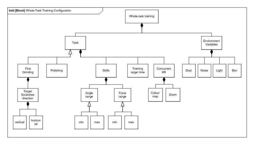
Figure 38. Features for the configuration of whole-task training.
