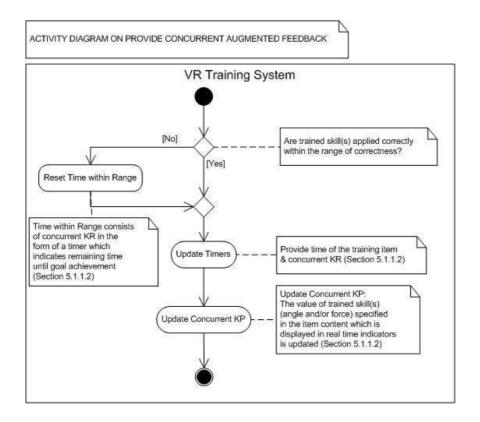
Figure 24. Activity diagram for providing concurrent augmented feedback in the form of KR and KP throughout part-task training.
