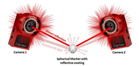
Figure 80. Example of tracking of a marker using two IR light emitted cameras
