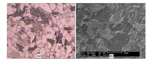
Figure 15. A metallographic replica correctly performed analyzed with (a) the light optical microscope and (b) the scanning electron microscope.
