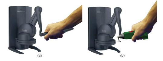
Figure 46. Handling of a Phantom Desktop as proposed in chapter 7, and mapping of the virtual precision rotary tool on the stylus of the haptic device (The body of the power tool in figure b. has been added with an image editing software).
