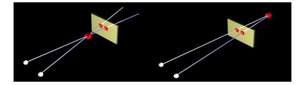
Figure 78. Perceived depth in front of and behind the display panel as a function of the representation of binocular cues and eyes convergence.
