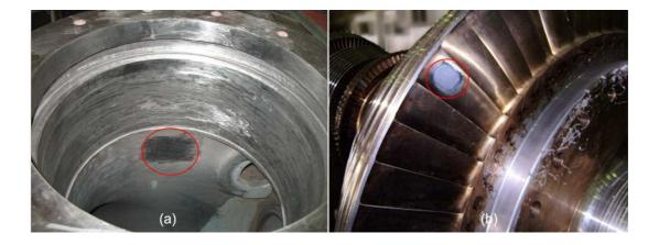
Figure 8. (a) Interior of an industrial valve and (b) a turbine blade on which metallographic replica tasks are commonly carried out.
