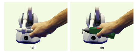
Figure 61. Handling of the haptic device and mapping of the virtual precision rotary tool on the device. The stylus represented the body of the virtual tool with the accessory attachment sitting at a  $90^{\circ}$  angle from the end of the stylus (This figure has been manipulated with an image editing software).
