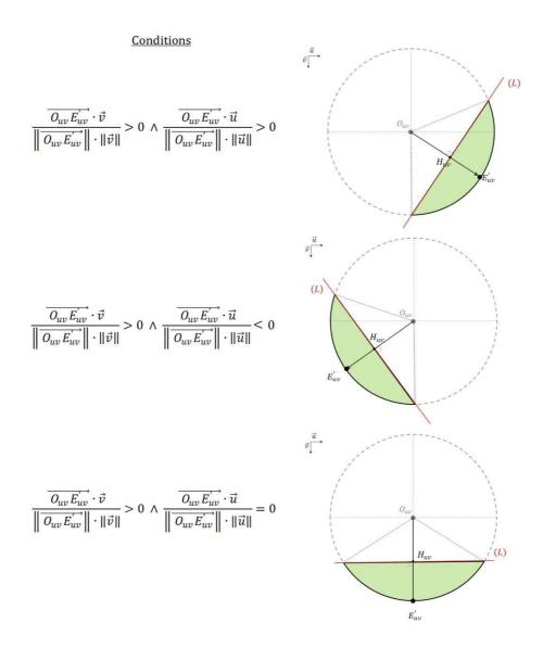
Figure 53. Case 1: representation of the circular segment area on the colour map. Percentages of task completion corresponding to pixels enclosed in that circular segment area are updated.
