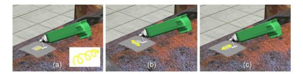
Figure 64. During the practice step, all participants were presented three trajectories: (a) circular, (b) forward to backward and (c) left to right. In exercises 6 to 10, FT were required to practice angle and force skills moving the virtual polishing tool across the metallographic replica area according to these trajectories.
