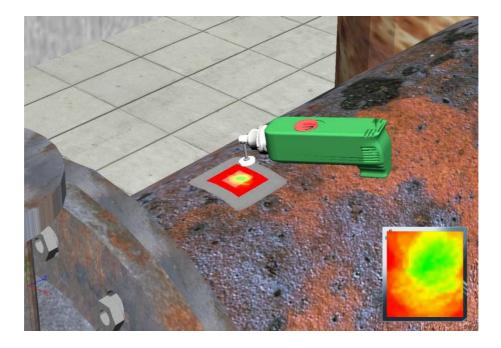
Figure 63. A trial of whole-task training supported the evaluation of the performance of a whole polishing task in a virtual environment. A colour map displayed on the area being polished enabled monitoring in real-time the advancement of the task. That colour map was also magnified and displayed in a panel located on the right lower corner of the monitor.
