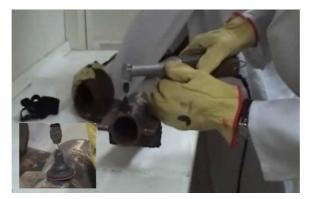
Figure 11. Precision rotary tool with right angle attachment equipped with abrasive flap disc to perform fine grinding operations.
