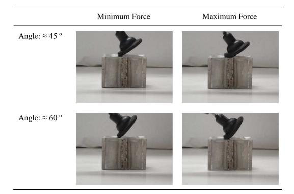
Table 7. Definition of the contact model in the form of a percentage which states for the ratio  $\delta$  of the diameter of the tool disc in contact with the material surface.
