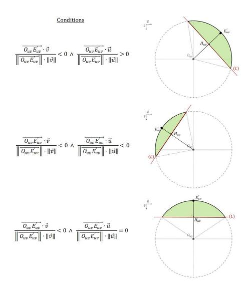
Figure 54. Case 2: representation of the circular segment area on the colour map. Percentages of task completion corresponding to pixels enclosed in that circular segment area are updated.
