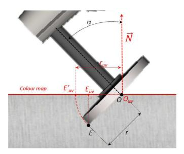
Figure 52. Normal projection of the point *E* on the colour map as  $E_{uv}$  and representation of the point *E* on the colour map as the edge point  $E'_{uv}$ .
