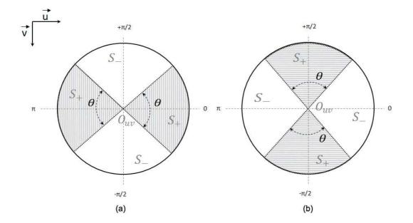
Figure 56. Circular sector areas  $S_+$  in which scratches are generated in the desired direction: (a) vertical and (b) horizontal. Sectors  $S_+$  are defined by a central angle  $\theta$  which has been heuristically set to 80° (Section 5.1.2.3).
