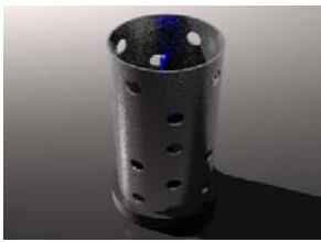
The whole sprue structure is place in a steel canister
