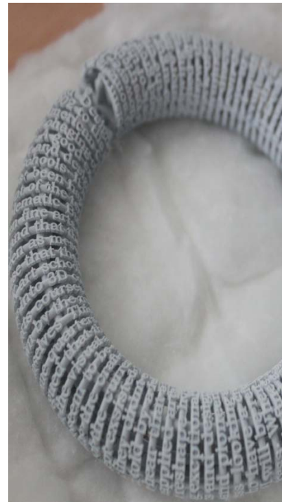
Wax Prototyped spiral sprue with narrative (with support)
