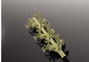
The plaster is washed away leaving you with a precious metal version of your original waxes
