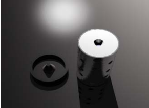
When the plaster is set, the canister is turned upside down and the rubber base removed. This reveals the bottom of the central wax sprue.
