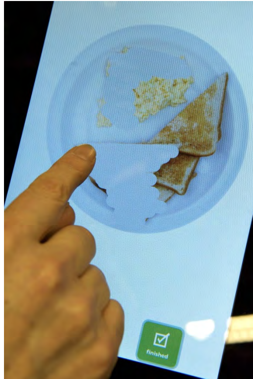
Figure 3: The user 'wipes away' food items eaten based on a visual assessment. The app is linked to a nutrition database calculating nutrients and calories consumed.
