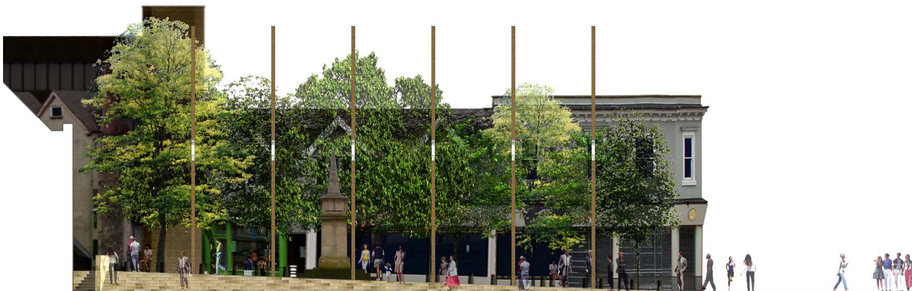
Section through site, at competition stage, showing tilted plane to retain archaeological remains and provide access to buildings to the north of the site.
