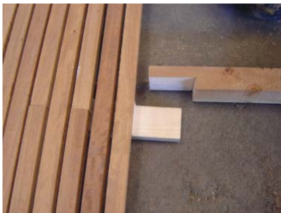
The development of a template to set out each panel of recycled Iroko strips in the contractor's workshop.
