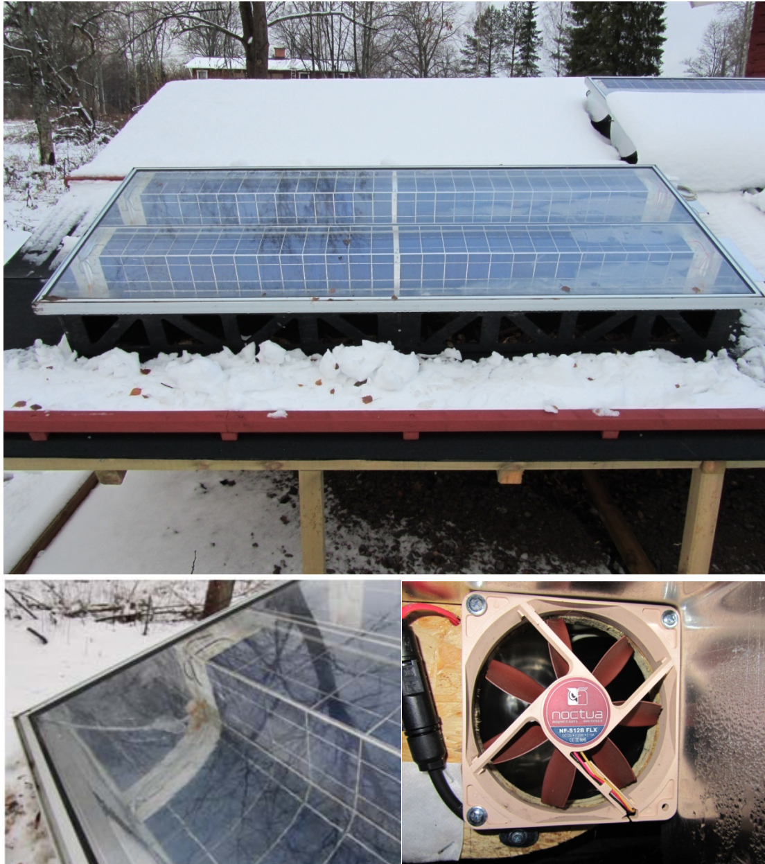
Figure 2: Ventiladed PV/T HR System Mock-up Equipped with a Fan and Solar Reflector
