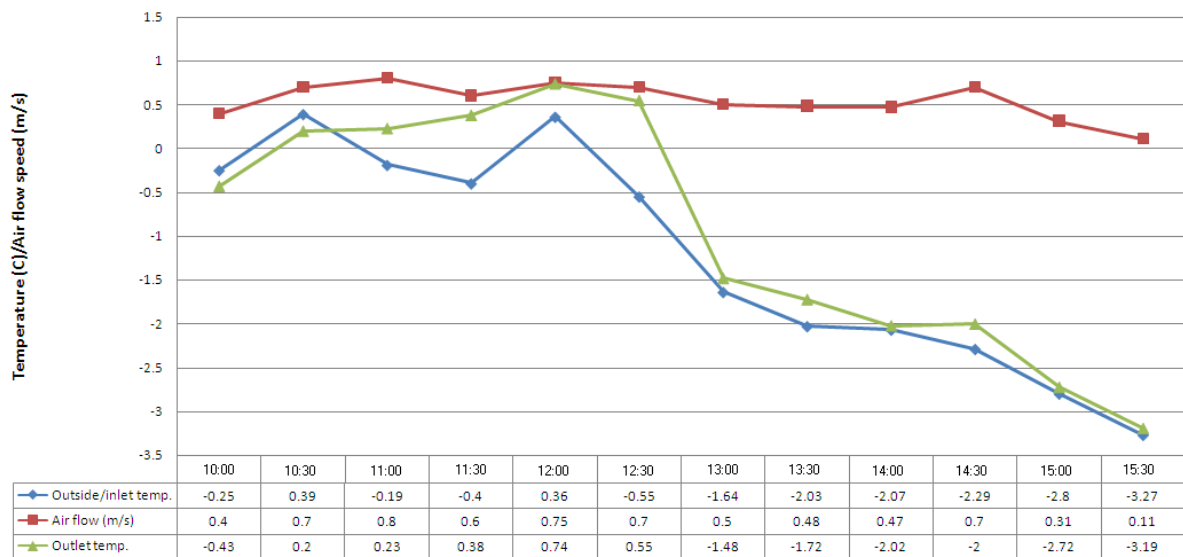
Figure 7: Inlet and Outlet Air Temperature and Velocity Monitoring Results of Ventilated PV/T HR Mock-up, 11 th November 2011
