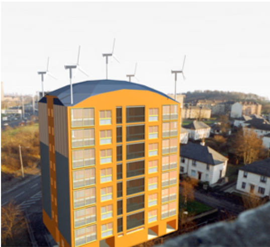
Figure 6: Domed roof form.
